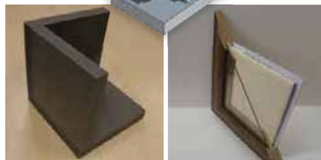
Plastazote® of various thickness glued to mountboard, for use as insert spacers for specialist framing
